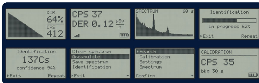
MS-PRD LCD screen captures: directional bar, CPS/DER readout, spectrum plot, identification and settings screens
